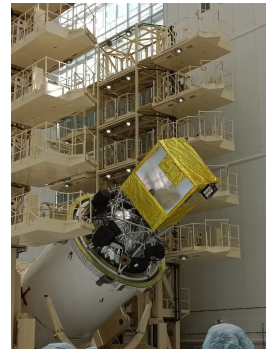
The process of preparing the launch vehicle for installation of the fairing
