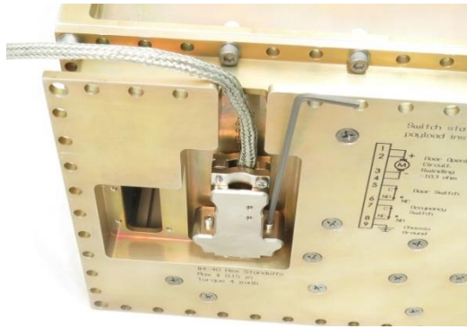
Figure 20-4: Installing CSD initiator electrical harness
