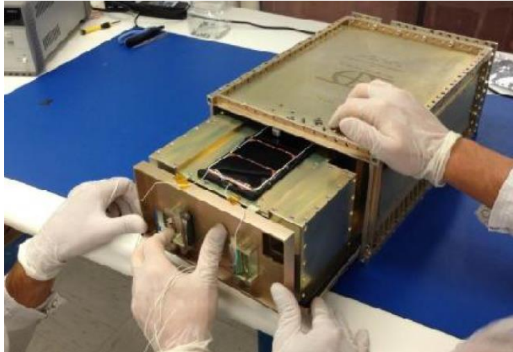
Figure 20-1: Installing 6U payload in CSD
