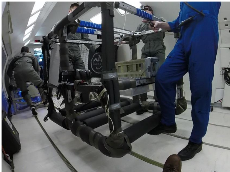
Figure 14-4: Test structure floating during micro-gravity test
