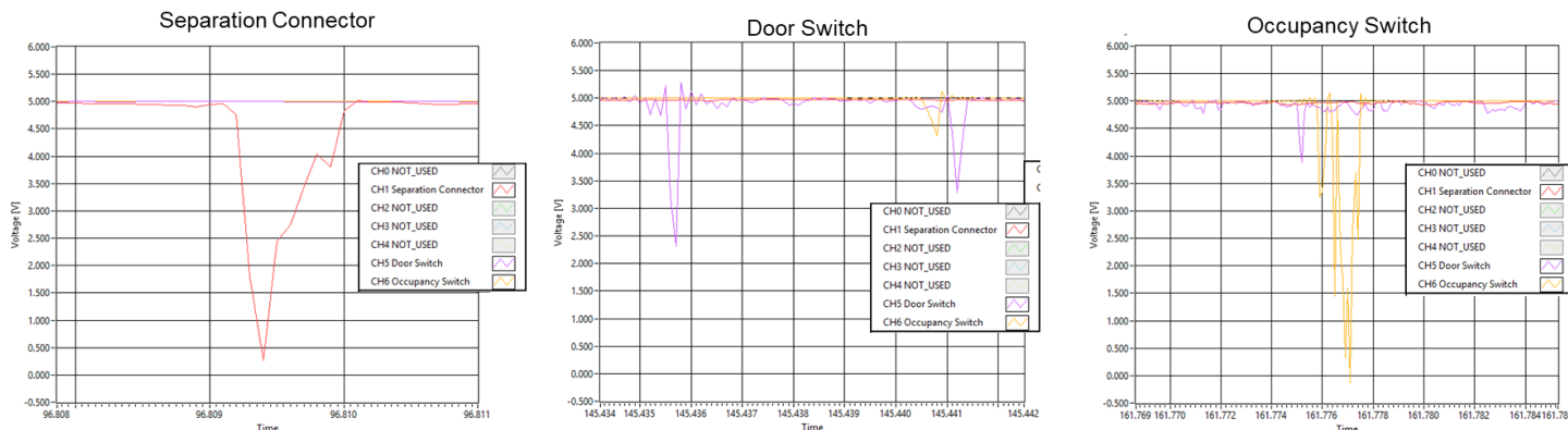
Figure 7-5: Typical duration of discrete intermittencies
