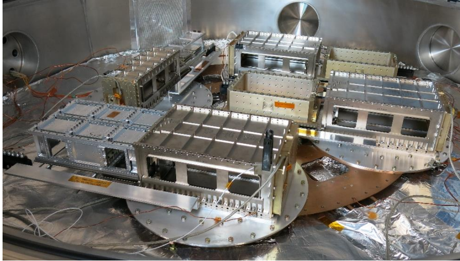
Figure 25-1: Four CSDs dispensing payloads onto conveyors in TVAC
