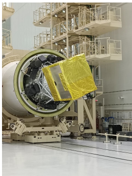
The process of preparing the launch vehicle for installation of the fairing
