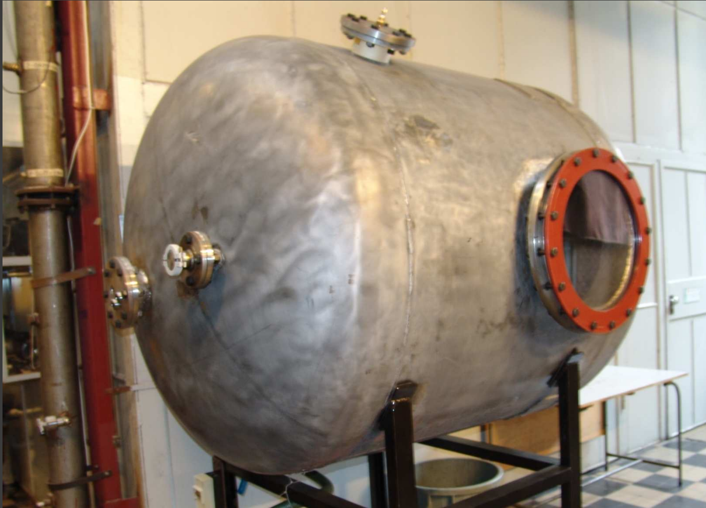
Vacuum tank prepared for test of the resisitojet
