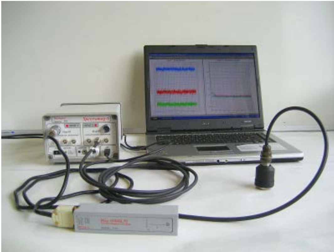
Figure 1: The Spectramag-6 system connected to a magnetometer and an accelerometer.
