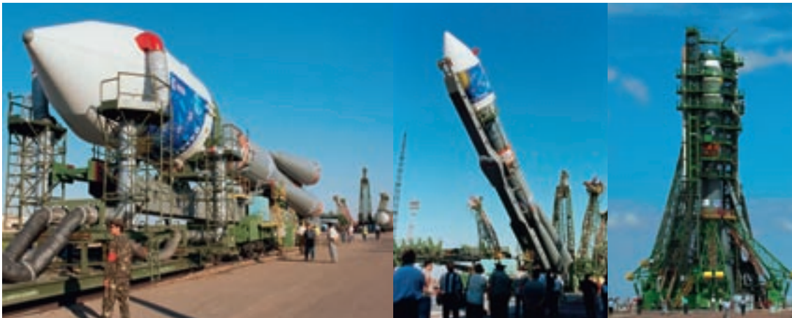
Figure 7-8: Launch Vehicle Transfer and Setup on Launch Pad.
