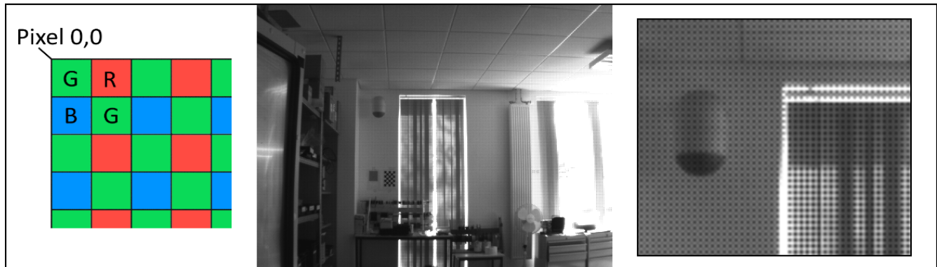
Figure 4: Left - The image sensor's bayer pattern. Centre - Raw image data displayed in 8-bit greyscale displays a subtle checkerboard pattern. Right - a zoomed-in view of the checkerboard pattern caused by the bayer filter.
