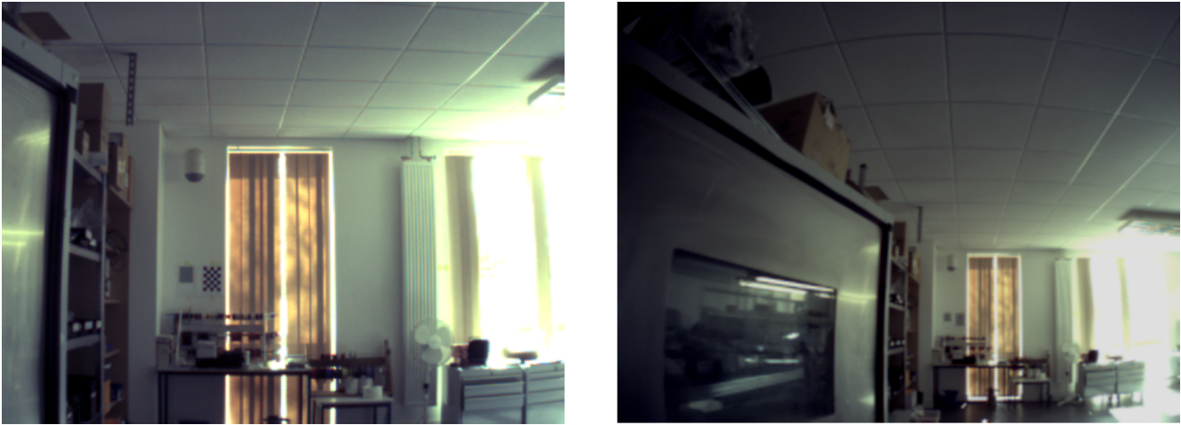
Figure 3: Example images taken in a lab environment with the two field-of-view parameter settings of the Capture command. The image on the left is a 480 x 360 full-resolution extract from the center of the image sensor's field of view (parameter 0x00), while the image on the right gives a FOV twice as wide by skipping every other pixel (parameter 0x01).
